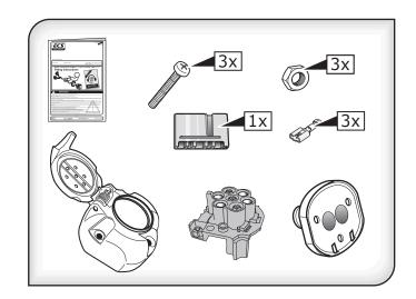
7 pin ISO socket with screw connection, 3 pin water-tight Cherry micro right side switch and mounting parts.
